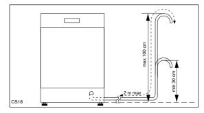
Likewise the internal diameter of the couplings used for connections to the waste outlet must be no smaller than the diameter of the hose provided.
